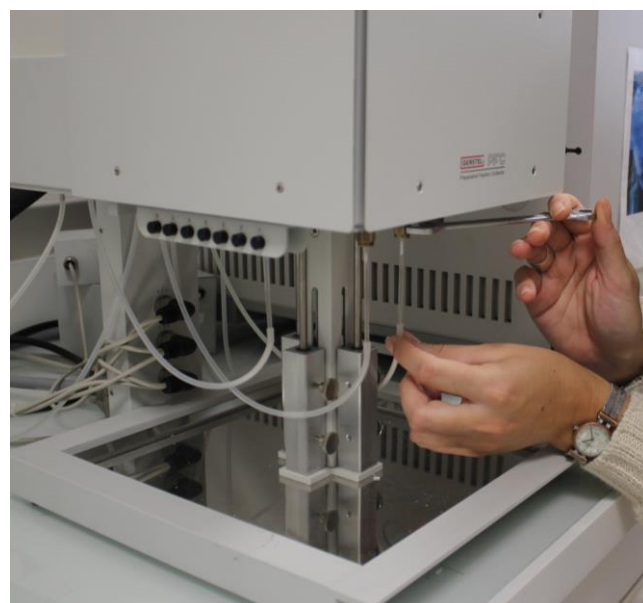
Figure : Fraction collector coupled with gas chromatography. The target compounds extracted from the ceramic matrix and are separated by chromatography from external contaminants then are trapped in the glass wool traps contained in the traps to be measured by the radiocarbon method.
